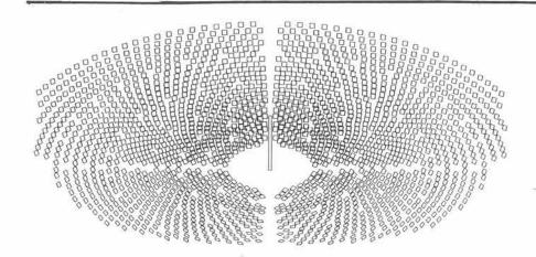
AS VIEWED FROM THE SUN at noon on Dec. 21, this is a field of 1760 heliostats looking at a central receiver. An output of MIR-VAL, the plot indicates this deployment's shadowing problems—note overlap left and right above the receiver.
